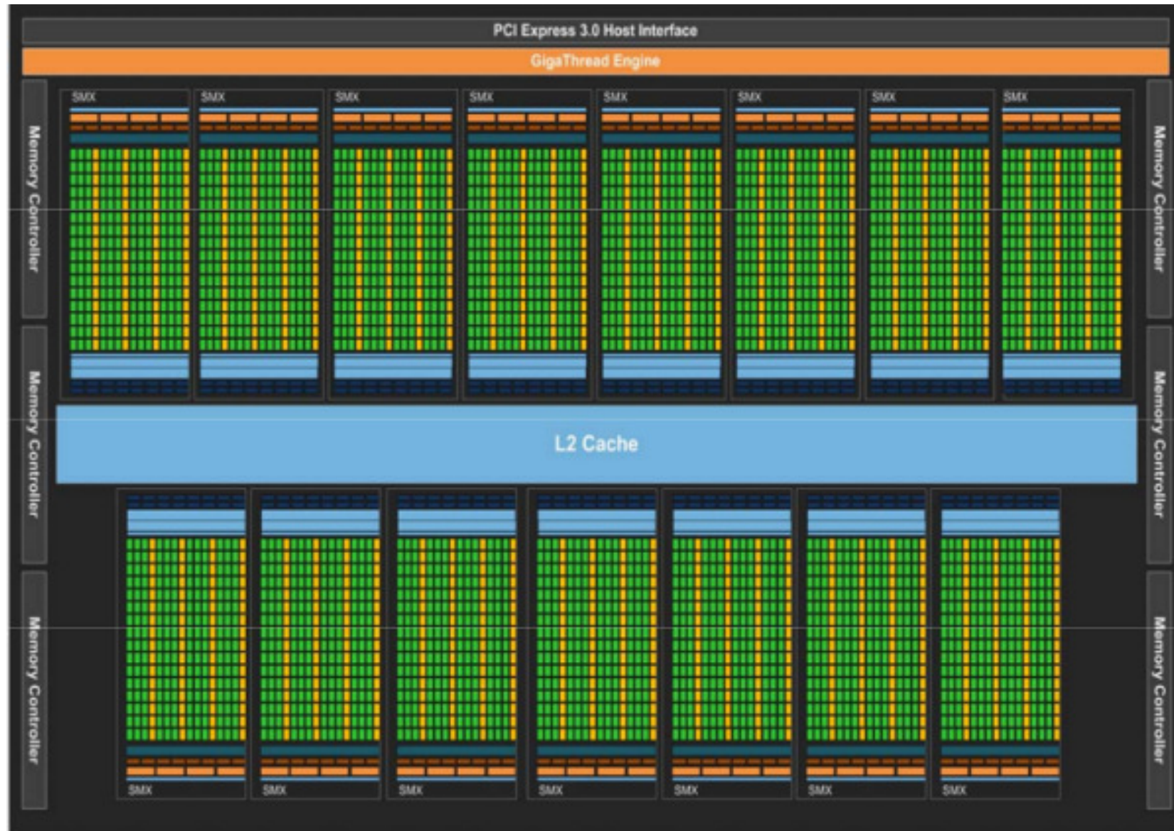
Nvidia's Kepler architecture as of 2012 (192 single-precision cores / 15 SM)
